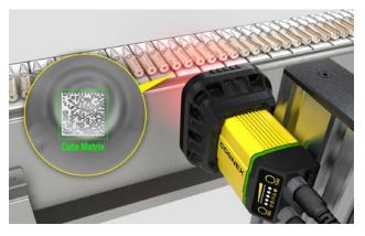
Serialization makes track-and-trace possible by requiring that every individual unit of a drug, in primary packaging, be identified with a unique serial and lot number and a matching GS-1 compliant barcode. Any secondary packaging has a corresponding serialized barcode that matches the codes on the primary packaging. Medical devices must also have a unique device identification (UDI) code.
