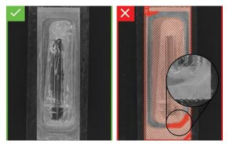
Conventional machine vision is extremely capable when dealing with consistent features, such as precision alignment, gauging, and 1D and 2D barcode reading. Deep Learning can solve previously intractable inspection and identification problems that involve visual distortions, reflections, ambiguity, and defect unpredictability.
